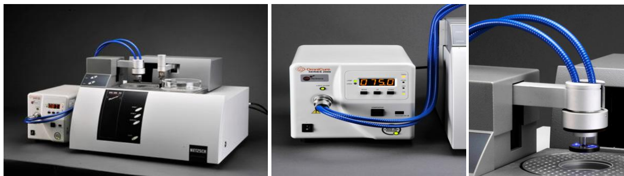
Fig. 2: NETZSCH photoDSC 204 FI Phoenix ® equipped with OmniCure S2000 Lamp
